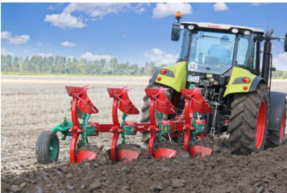
70/75cm underbeam clearance for the 150 S Variomat (80 cm for the 150 B Variomat) and 85/100cm interbody clearance for best performance in various soils and surface conditions.
