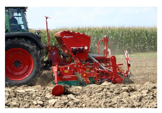
One of the main advantages for the operator is the constant depth control of the coulters, thanks to the direct link between the coulter bar and the roller mounted with a parallelogram linkage system – additional settings due to tine wear on the rotary harrow are not necessary.
