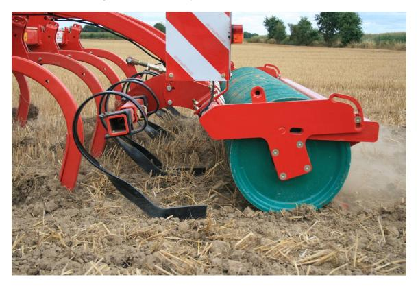
With the large range of rollers available, including the new Actiring and the Actipack, the CLC pro Classic can cope with all soil conditions and leave a weather-proof top layer or a firm seedbed with a surprisingly low power requirement.
